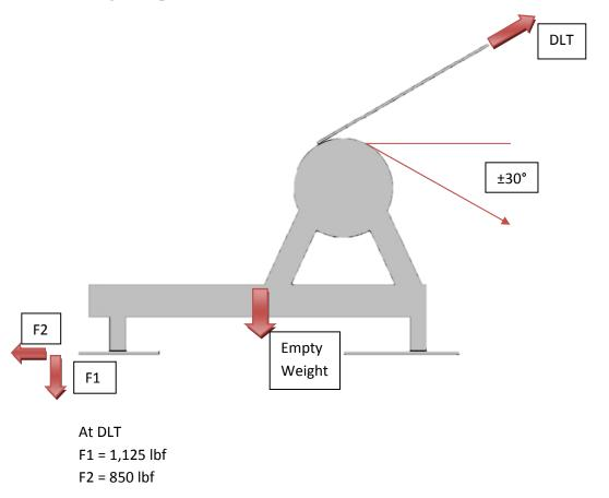
Forces are maximum forces per bolt, at DLT, for a 16 bolt hold down pattern (Rows spaced at 24", 72", and 96"). Analysis is good for a vertical fleet angle of  $\pm 30^{\circ}$  and a horizontal fleet angle of  $\pm 8^{\circ}$ .
